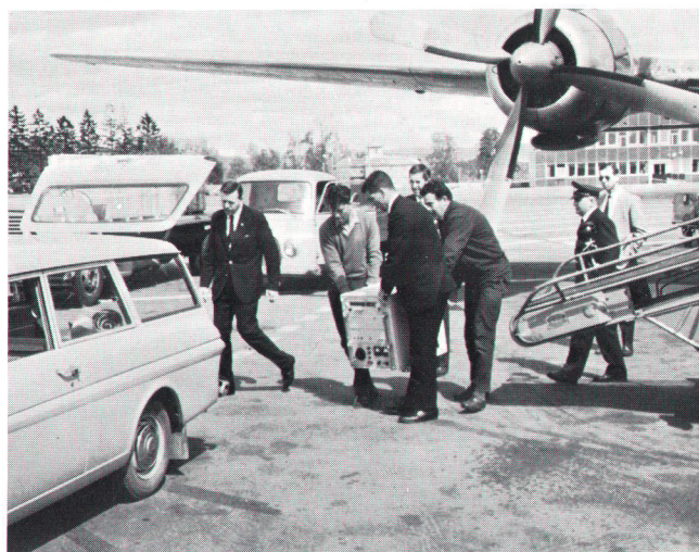
Fig. 2. Flying Clock No. 9, based on the -hp- portable cesium standard, arrives at Oslo, Norway, during 1966 time-synchronization trip. Clock was accompanied by Ronald C. Hyatt (c.) of -hp- Frequency and Time Division.
